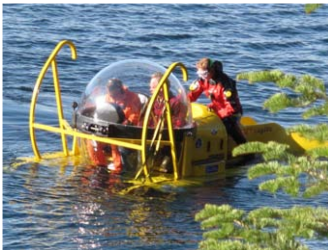
As Captain Cassell pilots, youth ambassador Sid Loomis works outside the submarine to adjust flotation before and after each dive.
